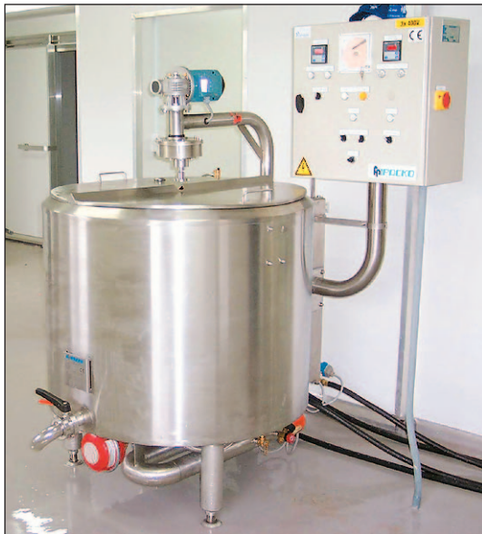
A Packo Fullwood batch pasteuriser can help create an on-farm processing plant.
